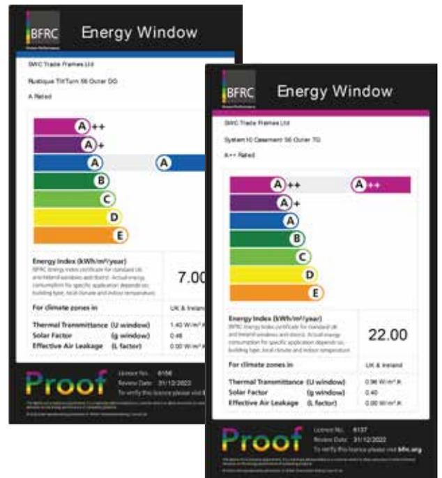
The energy labels are for reference only and apply only to specific PVCu products. The energy performance will change depending on profile and glass specification
